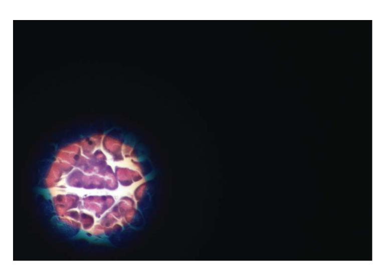
STEP 4 center the image using the two centering screws, so it looks like this: (Note centered, crisp edge)
